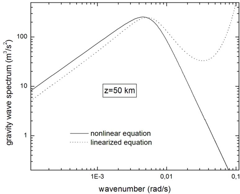
**Figure 3.** Gravity wave spectra calculated from Eqs 5 and 6 (solid line) and with linearized solution of Eq. (4) (dotted line) for the height  $z = 50$  km.
