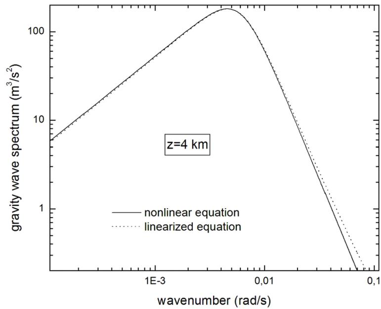
**Figure 2.** Gravity wave spectra calculated from Eqs. 5 and 5 (solid line) and with linearized solution of Eq. (4) (dotted line) for the height  $z = 4$  km.
